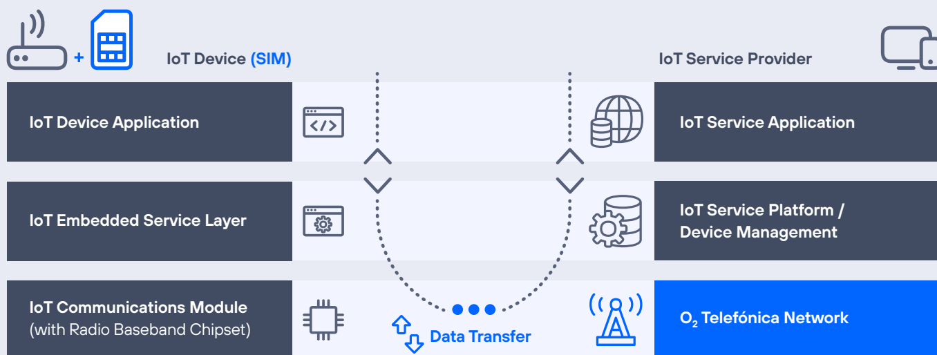
Figure 2: IoT Solution Layers, separate IoT Device Application and Service Enablement.
